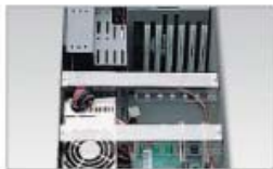
Two Adjustable Card Retainer Position
