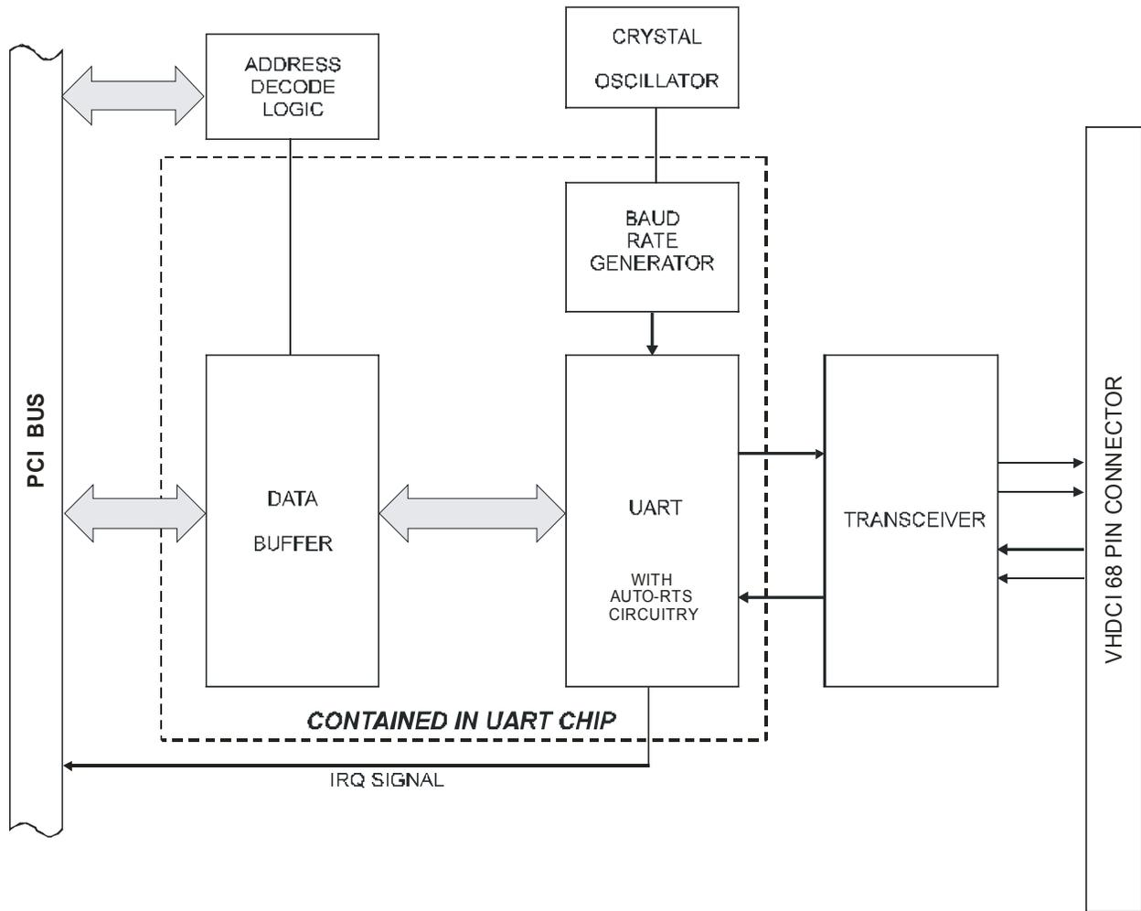
**Figure 1-1:** Block Diagram (Only one serial channel shown)
