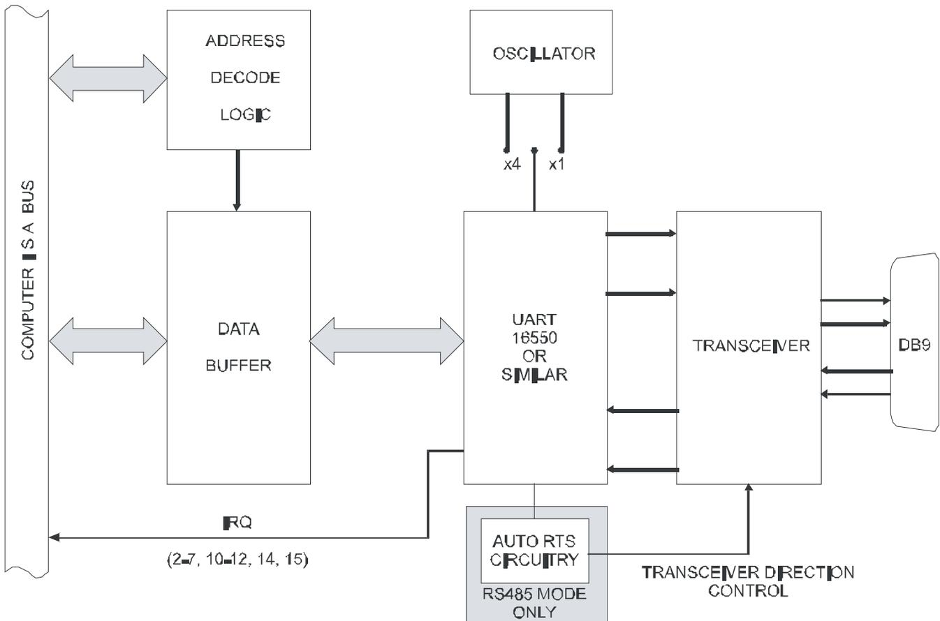
**Figure 1-1:** Block Diagram(Only one serial channel shown)
