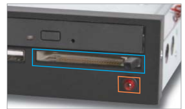
CF Reader and LED for HDD
