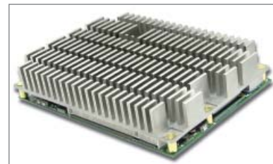
Passive Heat Sink
