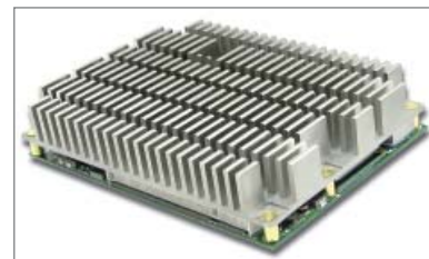
Passive Heat Sink
