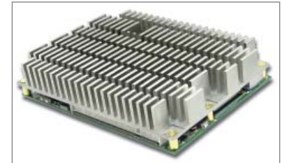
Passive Heat Sink
