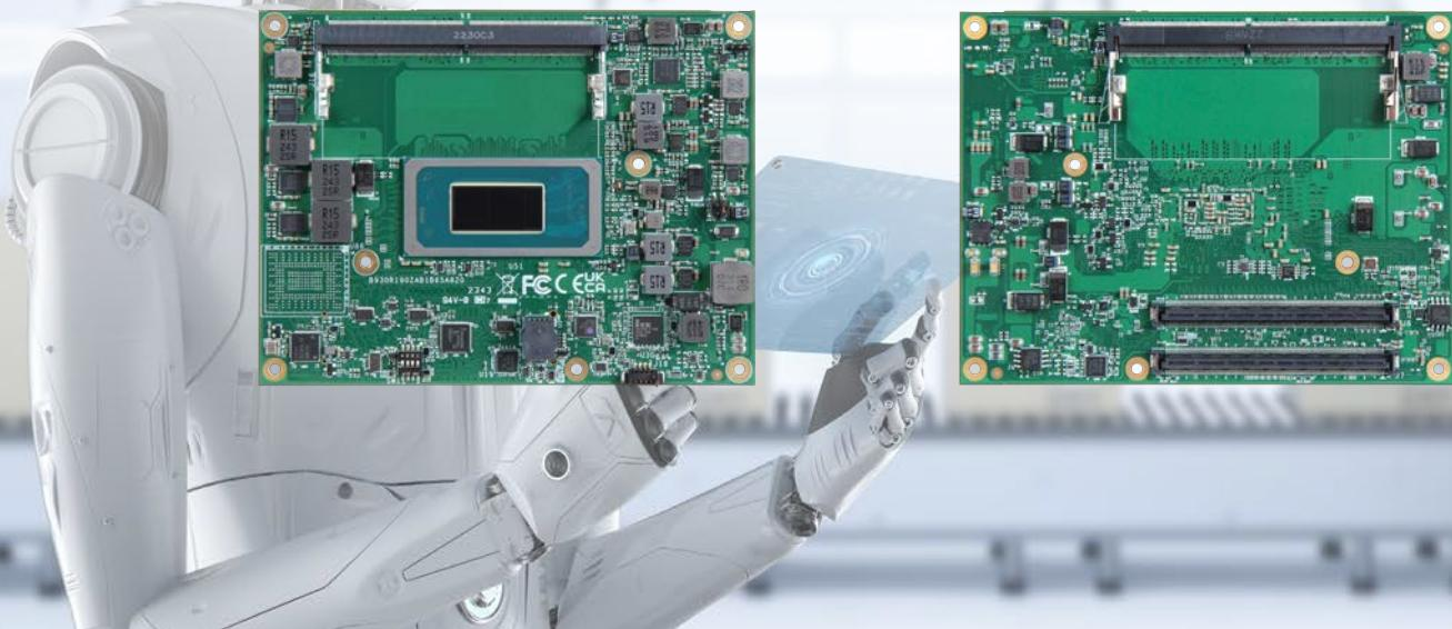
The PCOM-B65A is a COM Express Basic module (125 x 95 mm) designed for deployment in the core processing units of advanced humanoid robots. Although it draws more power than Atom-based modules (15W to 28W), the Intel® Core™ Ultra platform enables energy-efficient performance, even under limited cooling conditions.
