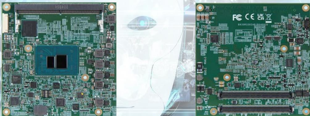
The PCOM-B646 is a COM Express Compact module (95 x 95 mm) designed for more demanding environments, with industrial temperature support ranging from -40°C to 85°C. It features robust thermal performance and supports up to 6x PCIe Gen3 x1 lanes, 4x USB 3.2 Gen2 ports, 2x SATA III ports., and Intel® I226 Ethernet. Display output via DDI, eDP/LVDS, and VGA enables multi-display support.
