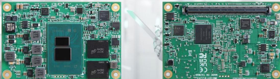
The humanoid robot market continues to demand high-precision, low-latency processing and seamless integration of diverse sensors. Portwell's PCOM-BA03, part of the COM Express® Type 10 family, offers a compact computing solution with a footprint of just 84 x 55 mm, ideal for integration into the head or torso of humanoid robots in space-limited embedded applications.
