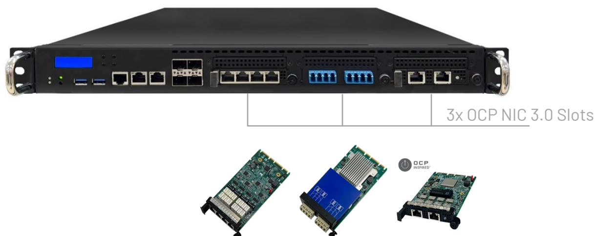
Figure 1. PNSR-5001 network appliance built with industry-leading design of three open standard OCP NIC 3.0 network interface cards with built-in bypass feature
